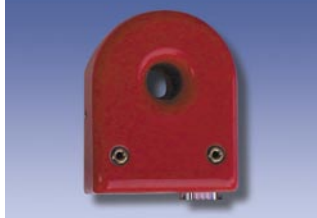
PSU600 Precision current transformer, max. 600A, u=1500:1 , DC to >100kHz, accuracy <(0.01%MV+0.005%MR)
