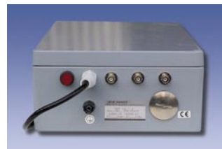
HST6-1, HST6-2, HST12-1, HST12-2 Precision high voltage divider for 6/12kV. Single pole isolated high voltage measuring (-1), dual pole isolated high voltage measuring (-2). Accuracy: 0.05% (45-65Hz), 0.3% (DC-100kHz)
