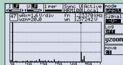
Measurement of the amplitude spectrum of the voltage harmonics in the HRM100 mode. An increase in the 47 th and 49 th , the frequency of the fundamental amounts to f_n/47=26.25\text{Hz}
